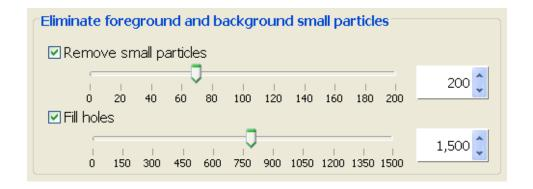
To eliminate background particles by size adjust the **Remove small particles** control. Particles smaller than the size selected in the control will be removed from the selection. To fill unselected areas inside vessels adjust the **Fill holes** control. To activate these controls click on their associated checkbox. The associated spinners can be used to dynamically modify the range of the controls. Remember to always consult the actual changes in the outline overlay of the test image.
