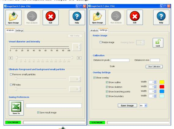
2. Open an image by clicking the **Open Image** button in the Analysis tab. AngioTool will open the image in a separate window and will perform an initial selection of vessels based on estimated parameters. The vessel selection is shown by a yellow overlay on the image. In order to tune the selection of the vessels the analysis parameters can be adjusted.
