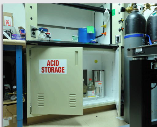
Store acids beneath the chemical fume hood.
