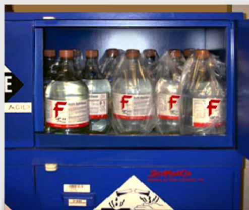
Store bases in a corrosive cabinet
