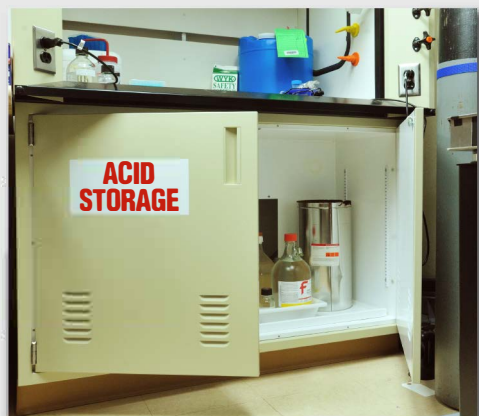
Store acid in a ventilated corrosive cabinet
